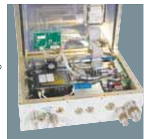
Interior view and typical bulkhead arrangement
